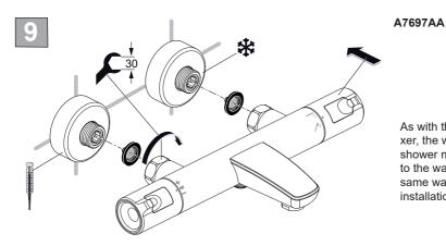
As with the bar shower mixer, the wall mounted bath/ shower mixer is assembled to the wall brackets in the same way to complete the installation.
