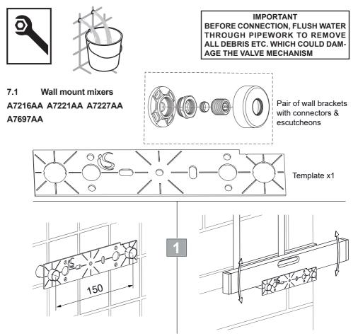
Ø15mm copper supply pipes should be run within the wall cavity. Hot supply pipe should be on the left hand side and the cold on the right.
