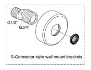
Pre-installation: Pipework should be run in or behind the solid wall, terminating with G1/2" female nipples securely fastened at 150 centres. To achieve a seal, apply PTFE tape (suitable for water) to the G1/2" threads of the S-connectors. Screw the S-Connectors into the nipples as shown, Use a spanner on the square flats if necessary.
