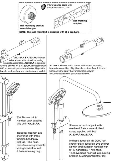
**NOTE: Shower kits** have to be carefully assembled during installation, chrome parts are packaged individually to prevent damage.
